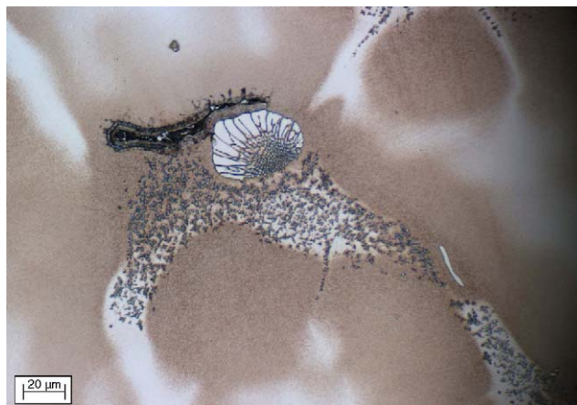
Fig. 2. Light optical micrograph of a directionally solidified sample of CMSX-4 interdendritic phases.
