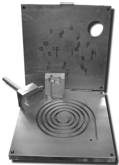
Fig. 6. Oil heated hot work steel mold with spiral cavity.
